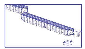
5. Connect drain channels, put end caps and outlet on. Join outlet with sewage pipe. Check the channel alignment. Before the concrete bedding dry's, lay channels with grates on concrete bed and level them. It is recommended that the channel's position should be 2-5 mm below the surface level, this guarantees optimal water collection.
